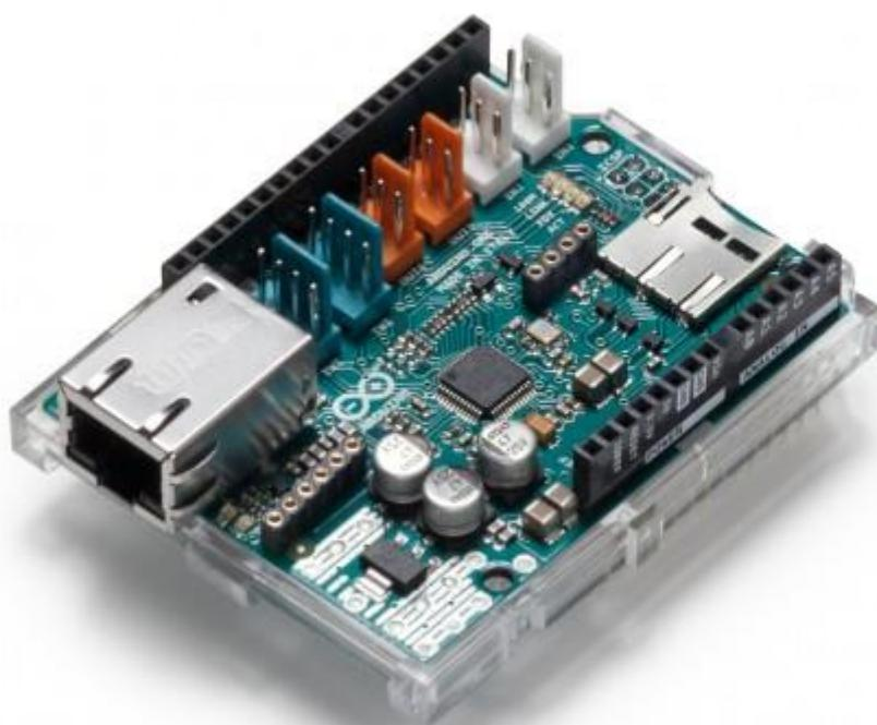
**Slika 3-2 Arduino Ethernet Shield**
